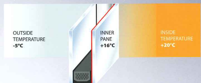
DOUBLE GLAZED UNIT using SGG Planitherm Total+
